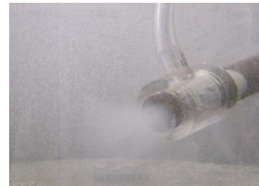
Fig. 1 Micro-bubbles generated by multi-fluids mixer.
