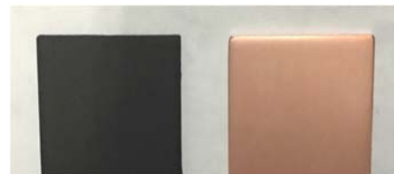
Fig. 2 Heat pipe walls before (left) and after (right) surface treatment
